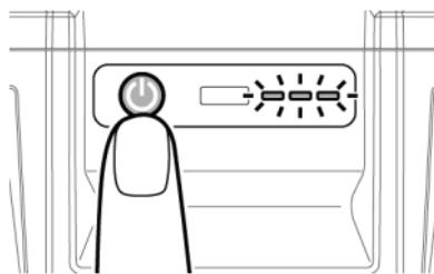
After TURNING ON, 3 small LEDs show the battery charge
