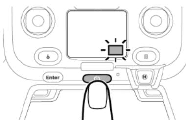
The icon on the lower-right shows the battery charge
